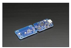
The Yocto-VOC-V3 device lets you estimate via USB the quantity of volatile organic compounds (VOCs) in ambient air, measured in CO2-equivalent ppm and TVOC. It also measures the ambient temperature and humidity. Measurements can be recorded on the internal flash for later retrieval when connected again by USB.
