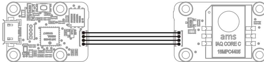
Wiring under the modules once separated.
