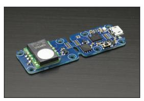
The Yocto-VOC-V2 device will let you estimate the quantity of volatile organic compounds (VOCs) in ambiant air via an USB connection, as well as record it on its internal flash for later retrieval when connected again by USB.
