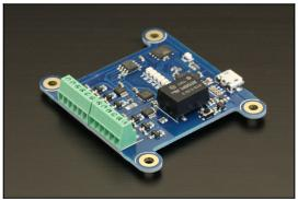
The Yocto-MaxiThermistor is a USB interface for NTC and PTC thermistors. It can measure up to six temperature points. Each of the six channels can be configured independently thanks to tables or reference temperatures and  $\beta$  coefficients. The Yocto-MaxiThermistor is an insulated device: there is an electric insulation between the sensor part and the USB part.
