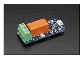
The Yocto-PowerRelay-V2 is a small USB power relay. It contains a USB-driven SPDT power relay switch: you can drive by software the relay input to one of the two outputs. To make it easier to test your project, two LEDs show the currently active output.
