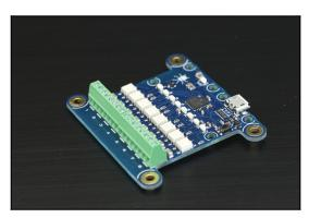
This USB device features 8 solid state relays, able to switch directly up to 48 VDC or 30 VAC r.m.s. for loads up to 1.3 A. Thanks to their onstate resistance of only 0.1 Ohm, they can even stand short peaks up to 5 A (max.100ms). This device therefore provides a compact alternative to mechanical relays for switching signals an small loads.
