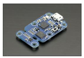
The Yocto-Light-V3 device is a USB ambient light sensor (lux meter) which allows you to measure ambient light up to 100'000 lux. Measurements can be read directly via USB or stored on the device internal flash for later retrieval when connected again by USB.
