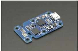
The Yocto-Light-V2 device is an USB ambiant light sensor (lux meter) which allows you to measure ambient light up to 65000 lux. Measurements can be read directly via USB or stored on the device internal flash for later retrieval when connected again by USB.
