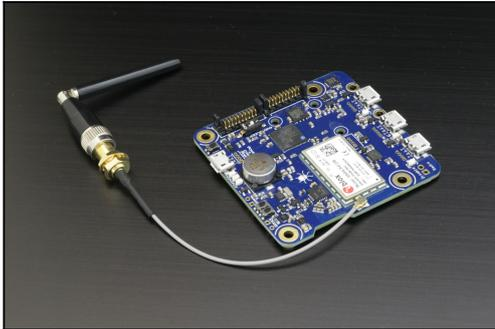
The YoctoHub-GSM-4G is a wireless-enabled module that can host three Yoctopuce modules to access them remotely through a 4G (LTE-M or NB-IoT) or 2G cellular network. It can be powered either by a Micro-B USB cable and a regular phone charger, or a 5V battery pack.
