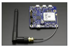
The YoctoHub-GSM-3G-EU is a wireless-enabled module that can host three Yoctopuce modules to access them remotely through a 3G GSM cellular network (UMTS and HSPA). It can be powered either by a Micro-B USB cable and a regular phone charger, or a 5V battery pack.
