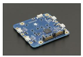
If you need to connect more Yoctopuce modules than allowed on our network hubs, you can add this extension board to them. Connected on the network hub with a picoflex ribbon cable (included), it allows you to connect 4 additional Yoctopuce modules to the network. There is no need for a separate power supply cable, as the shield is powered directly through the picoflex ribbon cable.
