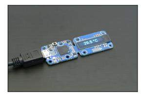
The Yocto-MiniDisplay is a very small 96x16 OLED display, driven directly from USB. It features a built-in controller which can render simple graphic objects, display text with various fonts, and even play pre-recorded animated sequences. Its small size makes it possible to use it for instance to display the individual status of each 1U server in a rack.
