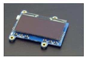
The Yocto-MaxiDisplay is a 128x64 OLED display, driven directly from USB. It features a built-in controller which can render simple graphic objects, display text with various fonts, and even play pre-recorded animated sequences. Since it requires no driver, it is ideal as a control panel for embedded applications driven by a mini-PC like a Raspberry Pi or MK802.
