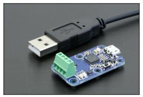
This device is a USB-controlled watchdog timer. When installed across a DC power cable, it can cut and restore the power whenever the control application fails to contact it.
