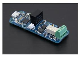
The Yocto-PWM-Tx can generate two distinct PWM signals using a frequency from 1Hz to 1Mhz. Signals can be generated in a variety of ways:
