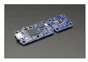
The Yocto-RangeFinder is a USB distance sensor (range finder). It works by measuring the time-of-flight of an infra-red laser beam that reflects on the target.
