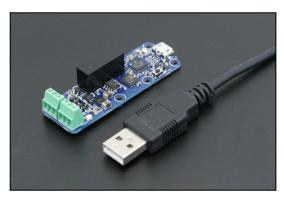
The Yocto-4-20mA-Rx device lets you read via USB the instant value returned by any industrial sensor following the 4-20mA standard, as well as record the measures on its internal flash for later retrieval when connected again by USB. The device can automatically map the current reading to a physical measure by applying a proportional rule. The module features two inputs, to connect two independent sensors.
