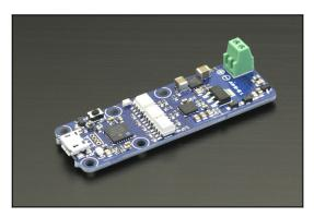
The Yocto-4-20mA-Tx is a USB 4-20mA signal generator. With this device, you can drive any other device featuring a 4-20mA input. This is an insulated device: the USB part is electrically insulated from the current loop part. The Yocto-4-20mA-Tx can drive any current loop powered from 12 to 24V with a 0.1% accuracy. Icing on the cake, the device can detect if the loop is properly powered or not.
