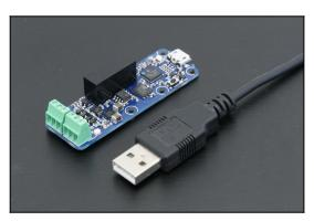
The Yocto-0-10V-Rx device lets you read via USB the instant value returned by any industrial sensor following the 0-10V standard, as well as record the measures on its internal flash for later retrieval when connected again by USB. The device can automatically map the current reading to a physical measure by applying a proportional rule. The module features two inputs, to connect two independent sensors.
