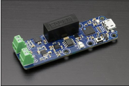
The Yocto-0-10V-Tx is a USB device with two channels that can generate independent voltages between 0 and 10V, for instance to control dimmable LED drivers. Each channel can drive up to 20mA.
