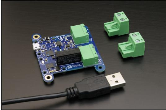
This device is a digital watt-meter allowing you to monitor the power consumption of electrical devices. It works with both AC and DC current. Regarding AC current, the device computes the real power consumption (not just the product of RMS voltage and current), so it can be used to monitor inductive loads. The Yocto-Watt can compute the power consumption during a given lapse of time. Accuracy is 1mWh, 1%.
