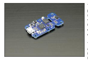
The Yocto-Proximity is a USB proximity sensor. It uses a pretty simple principle: the sensor part emits pulsed infrared light and measures reflection on nearby objects. Thanks to filters, ambient infrared light has very little effect on it, as long as the detector is not saturated. Beware, the sensor performance depends directly on the target color: a white object can be detected up to ~10cm, but a black and mat object can be detected up to ~2cm only.
