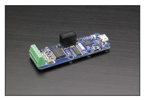
The Yocto-IO device provides 4 digital I/O, electrically insulated from the USB bus. Each I/O bit can be configured individually as a simple input, an open-drain input (internal pull-up), a TTL/CMOS-like output, or an open-drain output (open collector).
