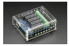
You need several USB relays in a tight form factor? The Yocto-MaxiPowerRelay controls 5 relays. Each of these relays can handle up to 250V and 5 Amp. The relay state is reflected by a LED. This module does not need external power, but the host computer or the hub to which the module is connected must be able to provide up to 250 mA.
