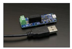
This device is a digital USB ammeter that allows you to measure current automatically. It can provide quite accurate digital measures (2 mA, 1%). It works with direct current (DC) as well as alternating current (AC) for which it provides the RMS value (5 mA or 3%).
