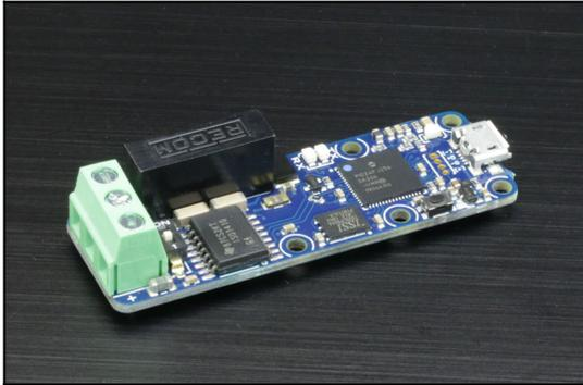
This device is a USB to RS485 adapter, that does not require a driver and does not install a virtual COM port.
