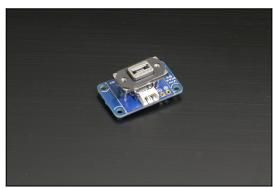
The Mini-Battery-Supervisor is a tiny circuit which makes it possible use a battery pack as power supply for low-power USB electronic appliances, while keeping the ability to connect a USB cable when needed.
