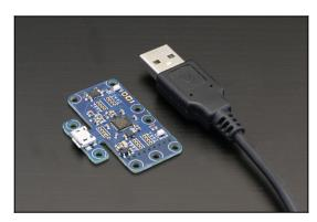
This device is a USB 2.0 hub. This is a multi-TT hub: it performs better than a regular single-TT hub when several USB 1.1 devices are connected to it. It is tiny (42x28mm) and its size can even be cut down to 36x20mm, most probably one of the smallest you can find...
