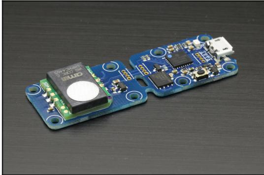
The Yocto-VOC-V2 device will let you estimate the quantity of volatile organic compounds (VOCs) in ambient air via an USB connection, as well as record it on its internal flash for later retrieval when connected again by USB.
