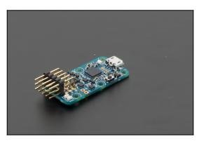
The Yocto-Servo device lets your software drive up to 5 RC servomotors through a standard USB interface.
