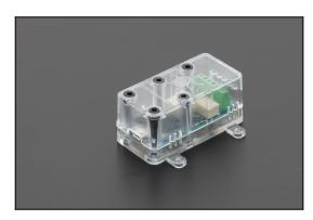
The Yocto-Relay device contains two USB-driven miniature unipolar relay switches. You can drive by software each relay input to one of two individual outputs (computer-driven switch). To make it easier to test your project, four leds positioned on the front side of the connector show the output currently active for each relay.
