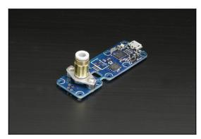
Do you need to monitor a pressurized circuit? The Yocto-Pressure might be the solution. This device can measure gas or liquid pressure up to 10 bars through USB. Moreover, it can record measured values on its internal flash for later retrieval when connected again by USB (built-in data logger). The Yocto-Pressure can also measure the temperature of the gas/liquid it is in contact with. The device features a SMC "one touch" fitting allowing to connect it to any 4mm tube very easily.
