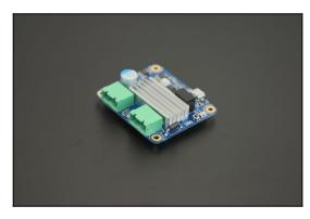
The Yocto-Motor-DC device is a USB motor controller (ESC) for brushed DC motors. It can make your motor go forward, reverse or even brake. Applied power is controlled by pulse width modulation (PWM) with a resolution of 0.1%.
