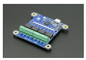
This USB device features 8 solid state relays, able to switch up to 160 VDC or 30 VAC, for small loads (up to 100 mA). It is an ideal solution to drive high-power relays. The state of each output is shown by a LED. This device does not require any external power.
