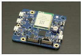
The YoctoHub-Wireless-SR is a wireless-enabled module which can host three Yoctopuce modules to access them remotely through a WiFi network. It can be powered either by a Micro-B USB cable and a regular phone charger, or a 5V battery pack.
