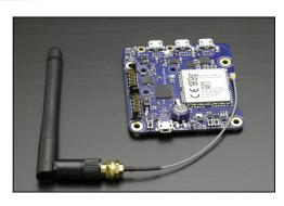
The YoctoHub-GSM-2G is a wireless-enabled module that can host three Yoctopuce modules to access them remotely through a 2G GSM cellular network (using GPRS EDGE, aka 2.75G). You can power it either with a Micro-B USB cable and a regular phone charger, or a 5V battery pack.
