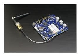
The YoctoHub-GSM-4G is a wireless-enabled module that can host three Yoctopuce modules to access them remotely through a 4G (LTE-M or NB-IoT) or 2G cellular network. It can be powered either by a Micro-B USB cable and a regular phone charger, or a 5V battery pack.
