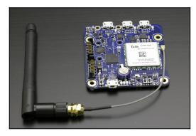
The YoctoHub-GSM-3G-NA is a wireless-enabled module that can host three Yoctopuce modules to access them remotely through a 3G GSM cellular network (UMTS and HSPA). It can be powered either by a Micro-B USB cable and a regular phone charger, or a 5V battery pack.
