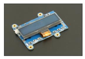
The Yocto-Display is a 128x32 OLED display, driven directly from USB. It features a built-in controller which can render simple graphic objects, display text with various fonts, and even play pre-recorded animated sequences. Since it requires no driver, it is ideal as a control panel for embedded applications driven by a mini-PC like a Raspberry Pi or MK802.
