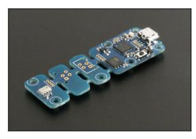
The Yocto-Altimeter device is a USB altimeter: it gives you an altitude estimate based on atmospheric pressure. The Yocto-Altimeter is sensitive enough to detect 25cm altitude changes. It also gives you the current pressure and temperature. Data can be recorded on the internal flash memory, in order to build a data history that can be retrieved later on over USB.
