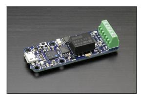
The Yocto-PWM-Rx is a 2 channel PWM input. Each channel can report frequency, duty cycle, and pulse length. It works from 0.05Hz to 250Khz and accepts any -30..+30V signal as long as it crosses the 0.7V threshold.
