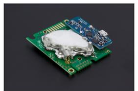
The Yocto-CO2 device will let you measure the quantity of carbon dioxide (CO2) in ambiant air via an USB connection, as well as record it on its internal flash for later retrieval when connected again by USB.
