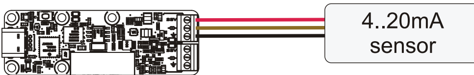
Wiring for a 3 wire sensor, powered by the Yocto-4-20mA-Rx-C (max. 80mA in all).
