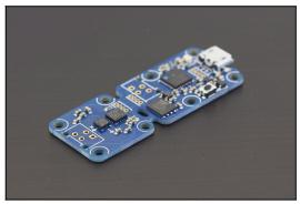
The Yocto-3D is a USB 3-axis accelerometer, gyroscope and compass. If you need to detect an orientation, a movement or a magnetic field, the Yocto-3D is what you need. This USB device provides a 3D accelerometer, a 3D magnetometer, a 3D gyroscope to measure angular velocity, a 2D inclinometer (tilt sensor), a tilt compensated compass and an inertial estimation of the orientation based on the 3D gyroscope.
