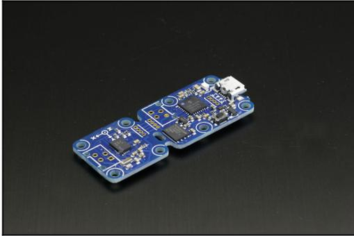
The Yocto-3D-V2 is a USB 3-axis accelerometer, gyroscope and compass. If you need to detect an orientation, a movement or a magnetic field, the Yocto-3D-V2 is what you need. This USB device provides a 3D accelerometer, a 3D magnetometer, a 3D gyroscope to measure angular velocity, a 2D inclinometer (tilt sensor), a tilt compensated compass and an inertial estimation of the orientation based on the 3D gyroscope.
