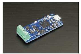
This device is a USB to SPI interface (master mode). It can handle the 4 standard SPI modes, and both bit encoding directions. It does not require a driver and does not install a virtual COM port.
