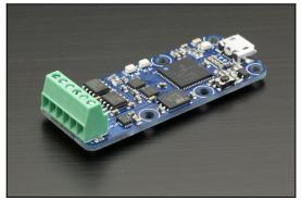
This device is a USB to serial adapter, similar to RS232 but it uses logical (TTL/CMOS) signal levels at 0/3.3V or 0/5V. It does not require a driver and does not install a virtual COM port.
