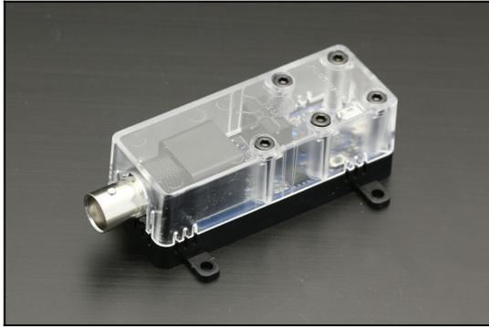
The Yocto-milliVolt-Rx-BNC device is a high accuracy USB voltmeter. It lets you measure by USB very small voltages (down to a few dozens of microVolts, and up to 2V max), even when they are generated by extremely weak sources (very high impedance). The BNC connector makes it possible to bring the signal using a shielded coaxial cable.
