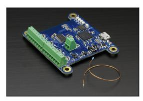
The Yocto-MaxiBridge is a precision ratiometric analog/digital converter to measure over USB the very weak voltage produced by load cells used in weighing scales, or any other type of strain sensor, or other sensor with a Wheatstone bridge output.
