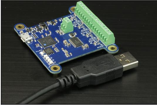
The Yocto-MaxiMicroVolt-Rx is a precision analog/digital converter to perform high-precision differential voltage measurements. The device provides 4 differential inputs, which are measured in round-robin loop. It provides a regulated 4.7V power supply. The inputs are not electrically isolated from the USB ground, but the inputs can freely float between the ground and the 4.7V supply: only the voltage difference between the two wires of each pair will impact the measured value.
